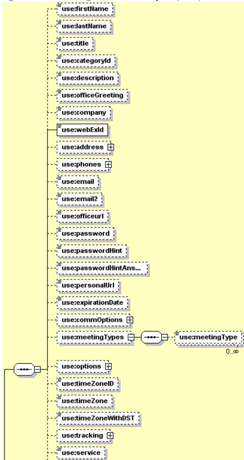
Figure 3-17 • Schema diagram for GetUserResponse (Part 1)
