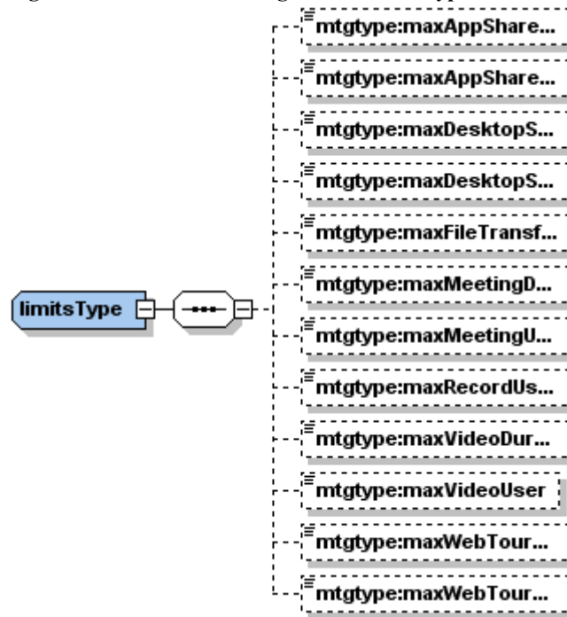
Figure G-130 • Schema diagram for limitsType
