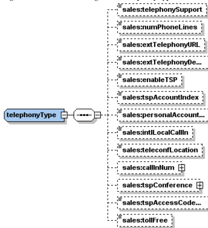
Figure G-116 • Schema diagram for telephonyType
