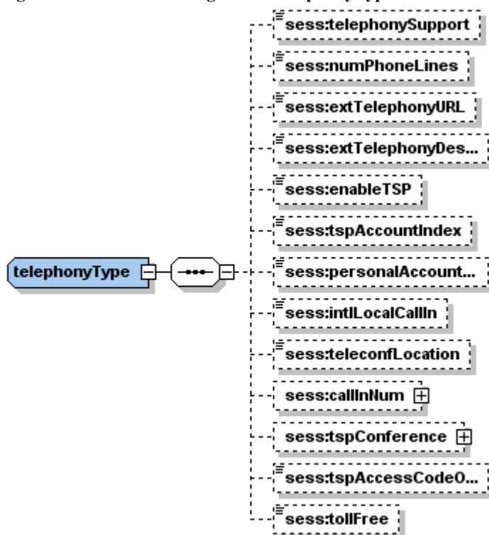
Figure G-65 • Schema diagram for telephonyType
