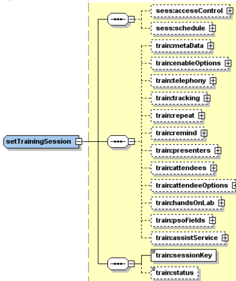
Figure 6-33 • Schema diagram for SetTrainingSession
